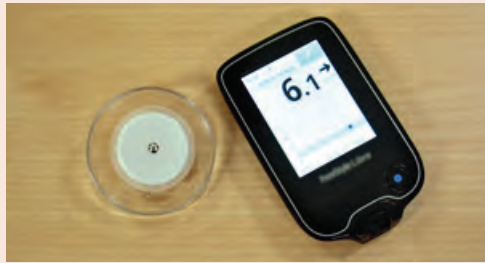
The flash glucose monitoring system, comprising a sensor (left) which is worn on the arm, and portable electronic reader (right).
